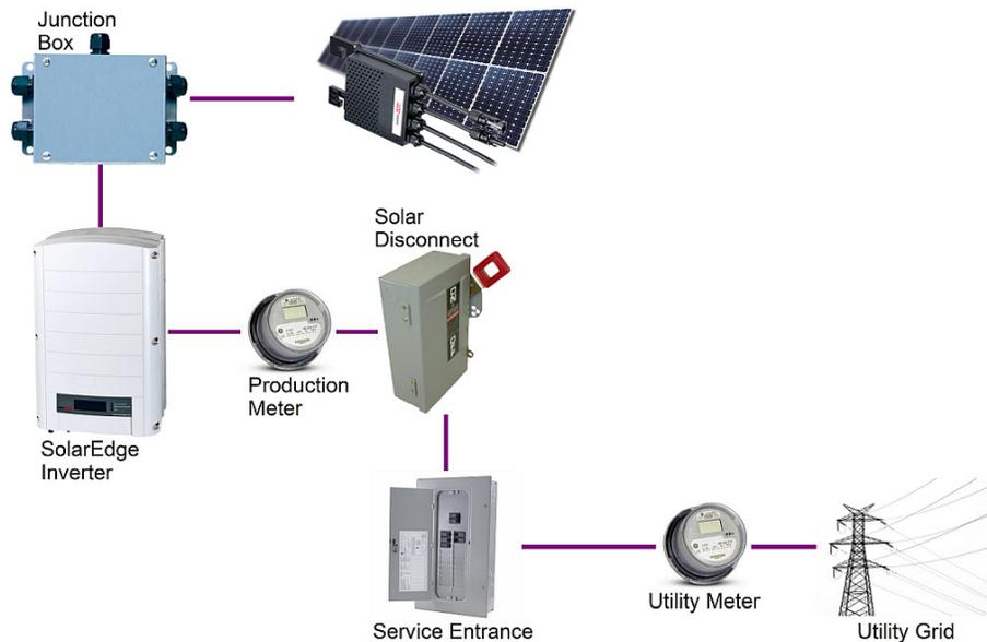
The SolarWorld modules each have an optimizer which is a DC-DC converter that maximizes the power available from that module. If some modules are shaded, the optimizers ensure that the remainder are not affected.
