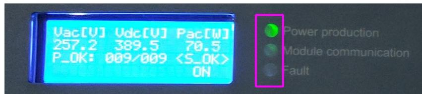
The top green LED indicates the inverter is on and making power. This is normal. The middle yellow LED flashes each time an optimizer talks to the inverter. The bottom red LED indicates a fault. If the fault LED is lit, contact mtvSolar and we will diagnose online and issue instructions accordingly.
