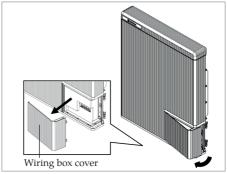
2. Open the wiring box cover (about 2~10 degree), and pull to remove it.
