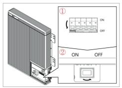
3. Turn off the battery pack by moving the circuit breaker switch ① to the OFF position.
