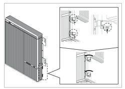
1. Press the two buttons and Pull the two latches (marked position) on the rear side of the wiring box cover. (hinged door)
