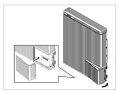
4. Close the wiring box cover, and lock the ratchet. And contact LG chem or your service provider.
